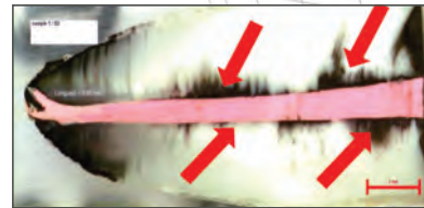
Dye penetration (black) after 30 days with Warm GP + PCS (Kerr)
