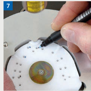
7 Mark out the selected drilling hole on used base plate (multiple usages)
