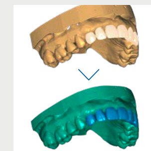
View of the shade gradient when nesting using Ceramill TruSmile
