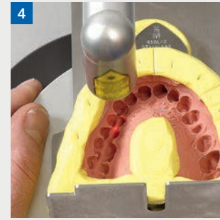
4 Position drilling hole with the aid of the laser beam and initiate drilling procedure
