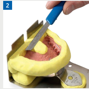
2 The impression is fixed onto the impression carrier with Giroform – putty, align the impression and putty insulation is trimmed
