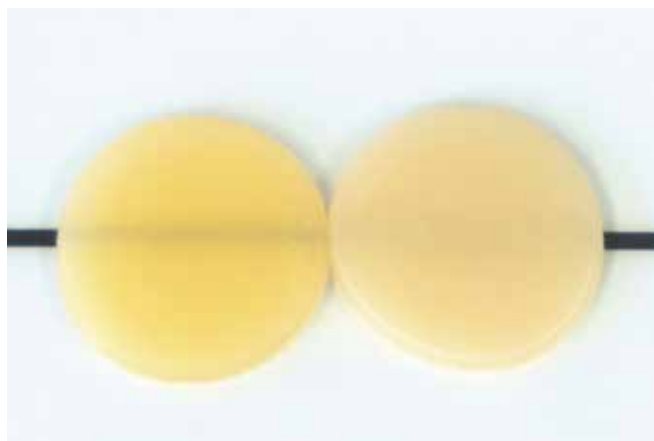
Disc specimen of GrandioSO Unlimited (Cluster-Shade A3) before the light polymerisation (left) and after light polymerisation (right)
