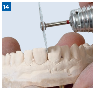
14 Partition/saw tooth arch into segments (Tip: in order not to damage the tooth arch, first separate the tooth arch in the middle)
