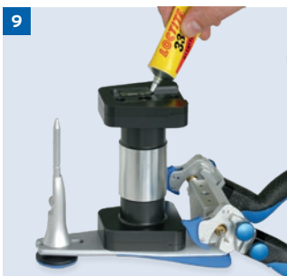
9 Apply two strands of glue near the center of the Splitex plate
