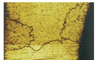
Coarse-grained structure of a conventional CoCrMo bonding alloy (magnification 100:1)
