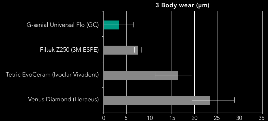
3-Body wear of various composite materials GC R&D, internal data, Japan, 04/2011. Data available on file.
