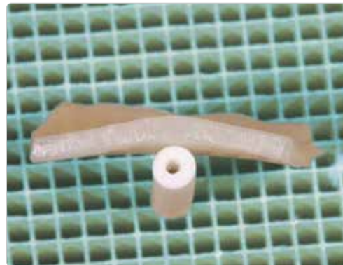
Results after 5th firing (770°C 1min, Hold). Test conducted by Masayuki Hoshi, RDT.
