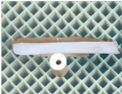
Results after 5th firing (770°C 1min, Hold). Test conducted by Masayuki Hoshi, RDT.
