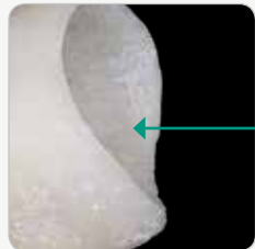
Reaction layer: Hybrid layer consisting of investment and press material
