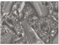
5a. Grandio† x5000 after 100,000 cycles. Note the gaps at the interface of the glass fillers and the resin matrix. Additionally, voids can be observed where fillers were lost.
