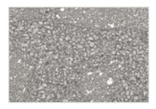
6a. KALORE x5000 after 100,000 cycles. Note the continuous interface between pre-polymerized fillers and the resin matrix.
