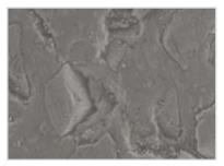
5c. Estelite Quick† x1000 after 100,000 cycles. Note that the interface between the pre-polymerized fillers and the resin matrix is no longer continuous and that the fillers are no longer an intrinsic part of the matrix.
