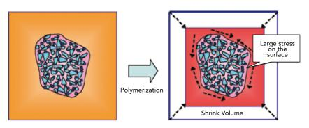
Figure 9b. Polymerization shrinkage stress with KALORE.
