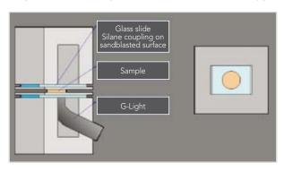
Figure 2. Three-body wear resistance test set-up.
