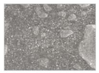
4a. KALORE x2000 after 100,000 cycles. Note the continuous interface between the pre-polymerized fillers and the resin matrix.
