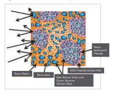
Figure 32d. Reflection in hybrid composites.
