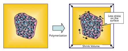
It can be concluded that DX-511, the new low shrinkage monomer, is effective in reducing shrinkage stress as demonstrated by testing of KALORE. The reduction in ongoing stress within the composite resin helps retain fillers in the matrix, especially after stress is applied to the cured composite resin. The surface smoothness, wear resistance and polish retention were also found to be superior with the addition of DX-511 to the composite resin formulation.
