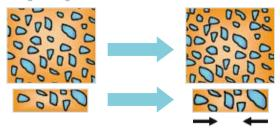
Figure 6b. Polymerization shrinkage of composites containing pre-polymerized fillers. Close contact between the pre-polymerized fillers prevents resin shrinkage.
