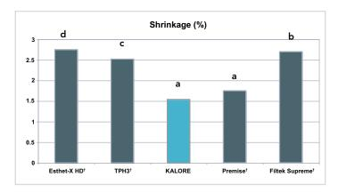
Figure 10. Volumetric Shrinkage.
