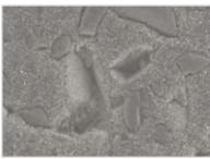
5b. Clearfil Majesty Esthetic† x1000 after 100,000 cycles. Note the loss of pre-polymerized fillers and gaps at the interface of the particles and the regin matrix
