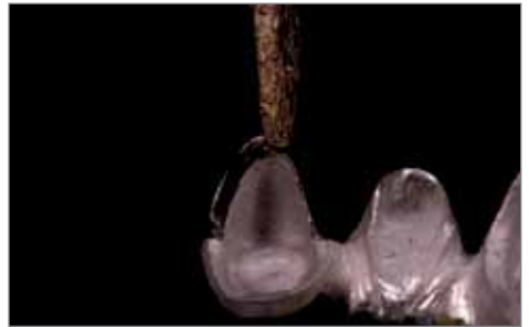
Fig. 37 The bulk of the metal is being trimmed using a coarser cut off disc.
