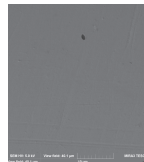
SEM image of a highly-polished surface showing a mirror-like image
