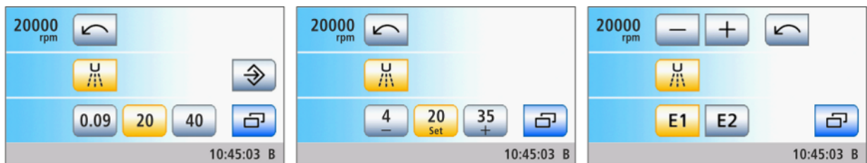
Motor dialog with fixed quick setting keys (left), programmable quick setting keys (center) and function levels (right)
