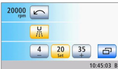
Motor dialog with fixed quick setting keys (left), programmable quick setting keys (center) and function levels (right)
